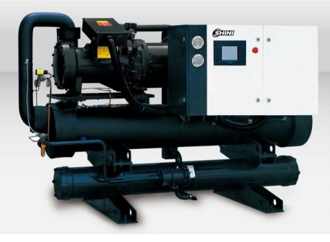
SICC-W series central water-cooled chillers adopt German-made BITZER with twin screw compressors, models with one or two compressors, suitable for using R22 and R134a refrigerants. High efficiency condenser and evaporator have been manufactured under national "BR1" standard. Featuring stable heat exchange and ease of maintenance, advanced controller with built-in microprocessor which gives better performance than single chip based unit.
