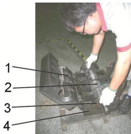
Picture 3-4: Installation of Bearing and Blade Rest 2
