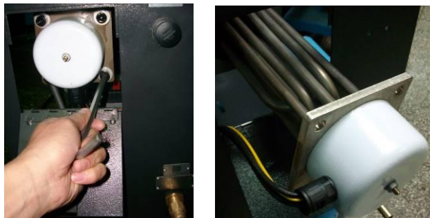
Picture 6-4: Heater Pipe 2
