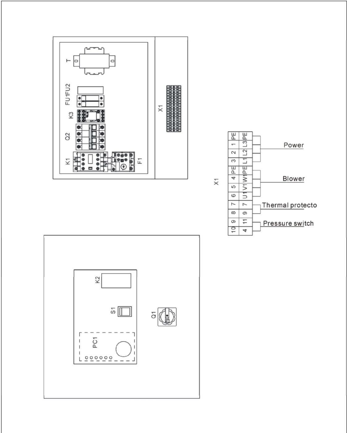
Picture 2-6: Electric Components Layout (SACC-3000)
