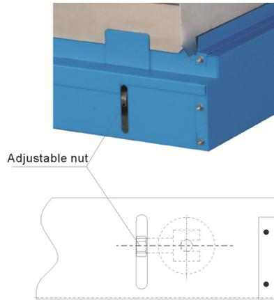
Picture 4-5: PVC Adjusting Drawing
