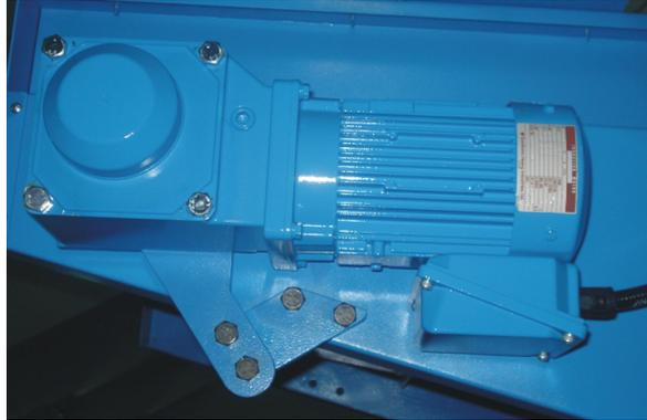
Picture 6-1: Gear Motor
