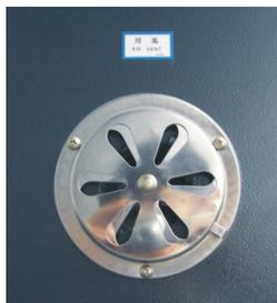
Picture 4-2: Adjustment of Air Rate
