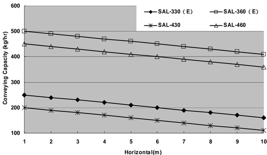
Picture 11-3: Performance Curve of SAL series (50Hz)
