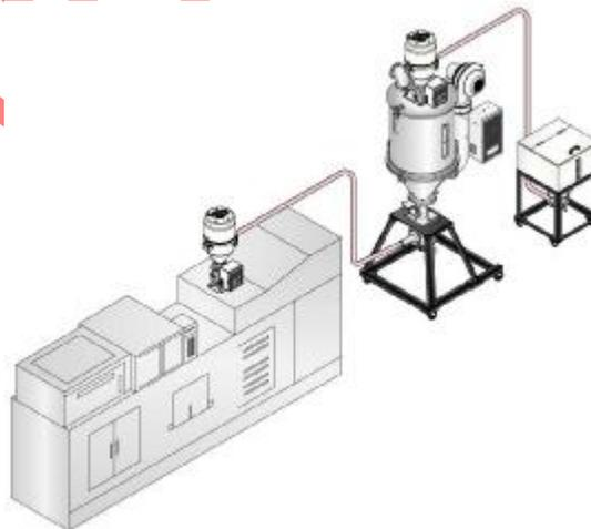
Picture 11-2: Installation on the Drying Hopper
