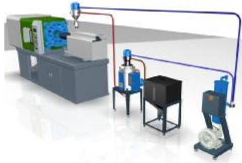
Picture 15-2: Collocation with Drying Hopper
