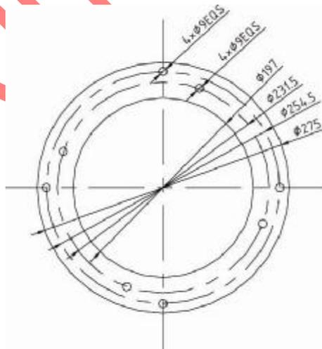
Picture 19-5: Dimension Chart for Base Installation of SAL-3U and Above
