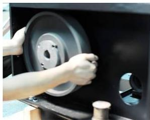
Picture 6-13: Installation of Belt and Belt Pulley 3
