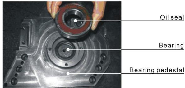
Picture 6-7: Installation of Bearing and Blade Rest 1
