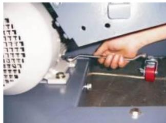
Picture 6-19: Installation of Belt and Belt Pulley 9
