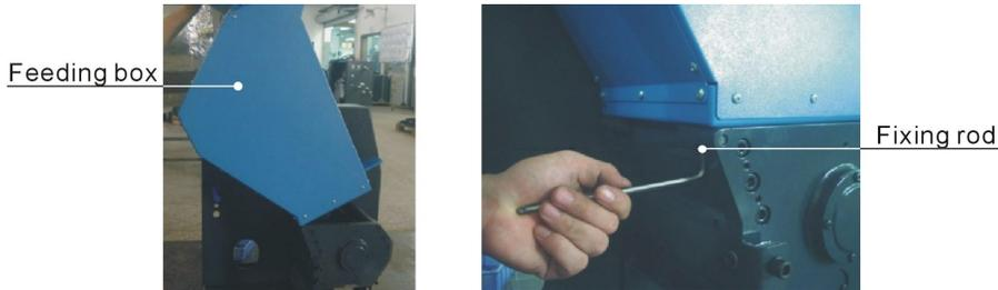
Picture 6-20: Installation of Feed Box and Feed Port 1
