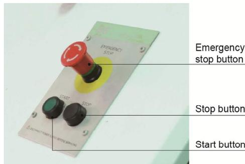
Picture 4-2: Stop, Emergency Stop and Startup button
