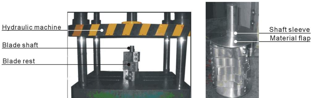
Picture 6-8: Installation of Bearing and Blade Rest 2
