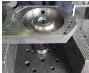
Picture 6-33: Step 3 to Take Out the Bearing
