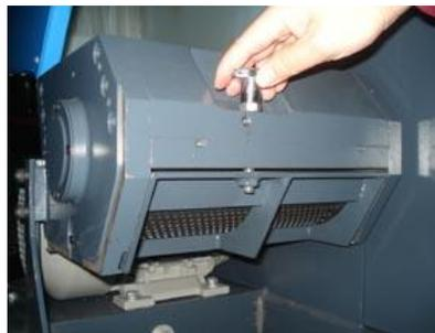
Picture 4-6: Open the Screen and Screen Frame 1
