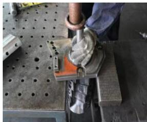
Picture 6-29: Step 2 to Take Out the Blade-rest Shaft
