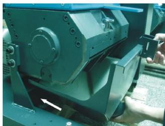
Picture 3-26: Installation of Material Collection Box 1
