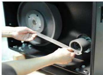
Picture 6-17: Installation of Belt and Belt Pulley 7
