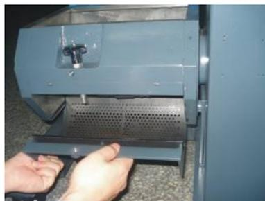
Picture 4-7: Open the Screen and Screen Frame 2
