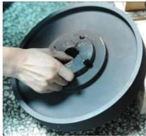
Picture 6-12: Installation of Belt and Belt Pulley 2
