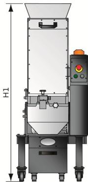
Height-increasing storage tank helps to collect and store regrind. Applicable to SG-16N/20N series.
