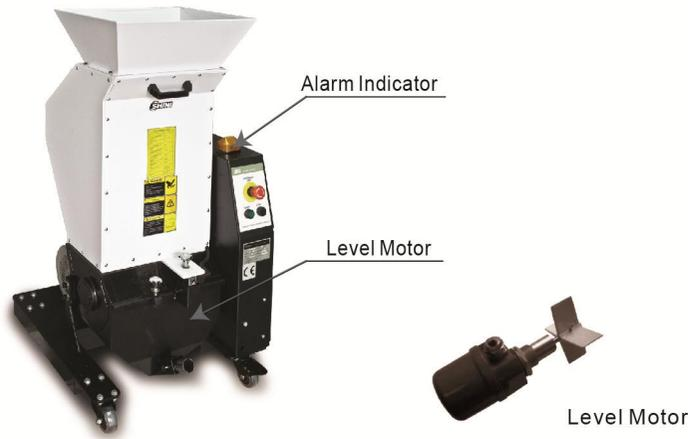
Full-receive alarm device can help to realize unmanned operation and no materials will be wasted. Whenever the regrind level reaches the motor position, the machine will be forced to stop and be cut off via its sensor, thus stop the granulator and warn the user by sounding an alarm. Applicable to SG-16N/20N series.
