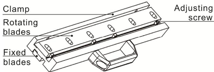
Picture 4-12: Blades Installation Adjusting (SG-20N)
