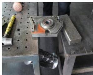
Picture 6-30: Step 3 to Take Out the Blade-rest Shaft
