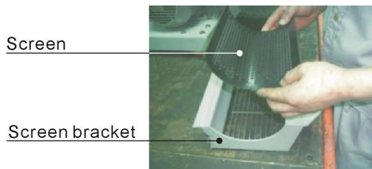
Picture 6-22: Installation of Screen and Screen Frame 1
