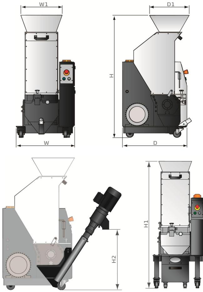
Optionally Equipped with Coiled Spring Conveyor
