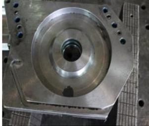
Picture 6-31: Step 1 to Take Out the Bearing
