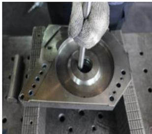
Picture 6-32: Step 2 to Take Out the Bearing
