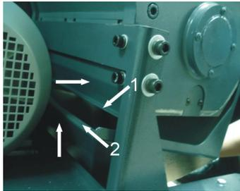
Picture 3-27: Installation of Material Collection Box 2
