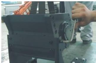
Picture 6-11: Installation of Belt and Belt Pulley 1
