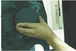
Picture 6-10: Installation of Bearing and Blade Rest 4
