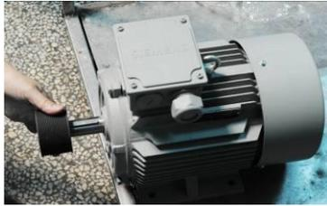
Picture 6-15: Installation of Belt and Belt Pulley 5
