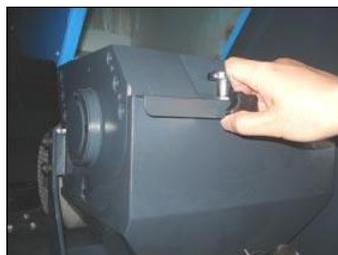
Picture 3-29: Installation of Material Collection Box 4
