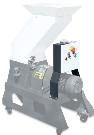
Picture 2-9: Control box with intermittent running function
