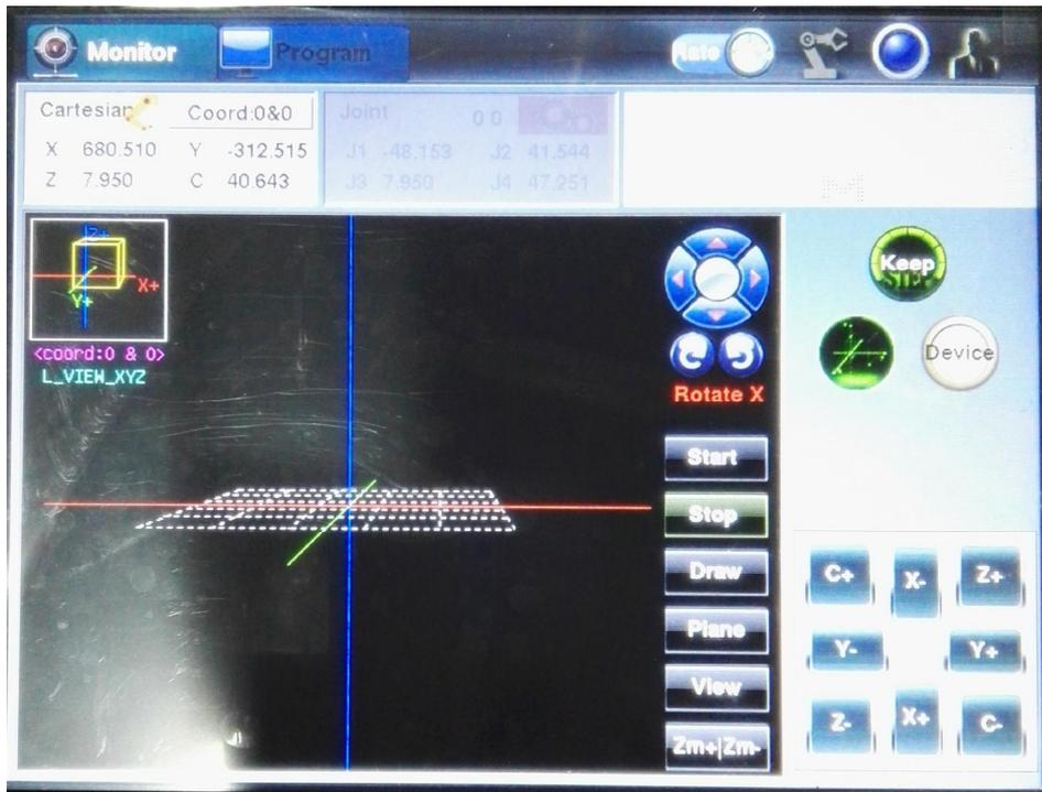
FlexPendant interface is shown in the graph above, based on customer's demand to set the parameters of the robot. The instruction of setting and usage could be found in "teaching pendant manual".
