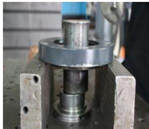
Picture 6-16: Step 1 of Bearing Dismantlement
