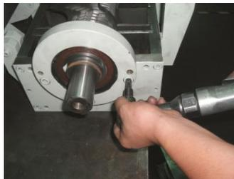
Picture 6-6: Installation of Bearing and Cutter Shaft 3
