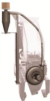
This device utilizes loading blower to convey regrind into the cyclone dust collector to separate the regrind from the air and then the regrind will fall into storage hopper or cloth bag.
