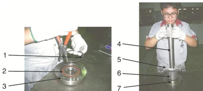
Picture 6-4: Installation of Bearing and Cutter Shaft 1
