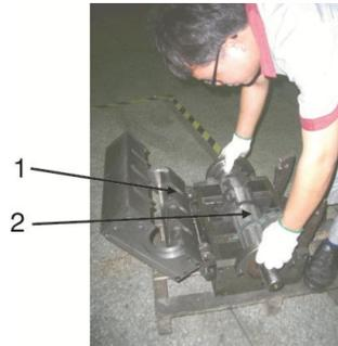
Picture 6-5: Installation of Bearing and Cutter Shaft 2
