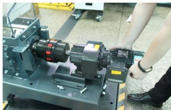
Picture 6-12: Step 1 of Gear box Dismantlement
