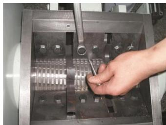
Picture 6-7: Installation of Teeth Cutter and Fixed Blade
