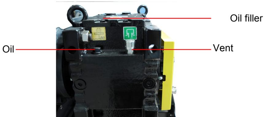
Picture 5-1: Oil Filler, Oil Pointer, and Vent
