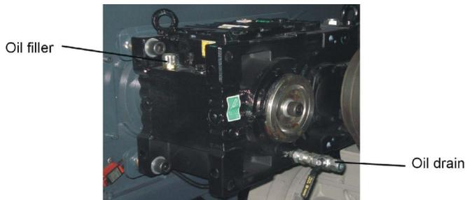
Picture 6-3: Oil Filling and Drain of Reduction Gear
