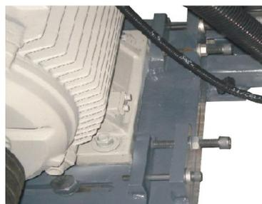
Picture 3-7: Installation of Main Cutter Shaft and Bearing 3
