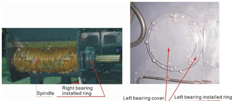
Picture 3-4: Installation of Main Cutter Shaft and Bearing
