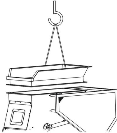
Picture 3-2: Installation of Feed Hopper
