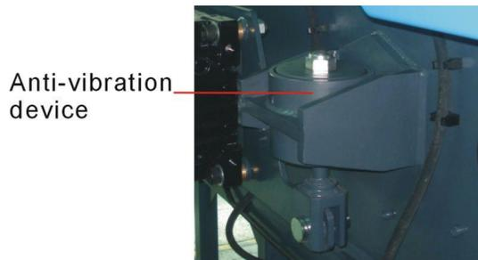
Picture 6-4: Anti-vibration Device
