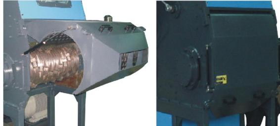
Picture 3-9: Sieve Net and the Installation of a Screen
