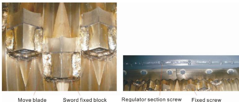
Picture 3-8: Installation of Fixed and Rotate Blades
