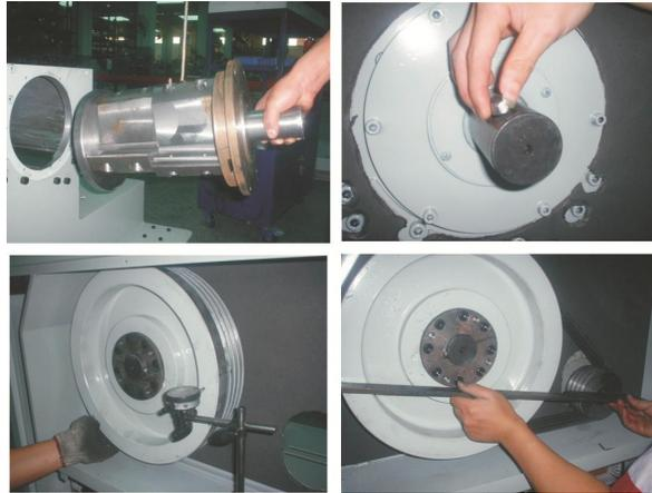
Picture 6-14: Installation of bearing, motor, belt Pulley and belt
