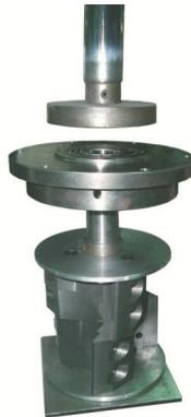
Picture 6-12: Installation of bearing block and bearing
