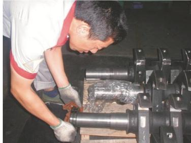
Picture 6-10: Installation of Bearing and Blade Rest
