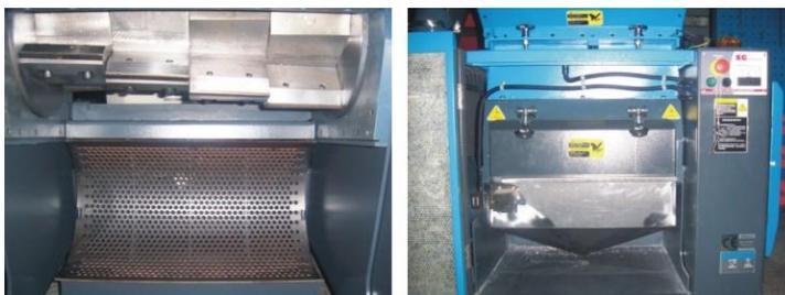
Picture 6-15: Installation of screen, screen bracket and storage box
