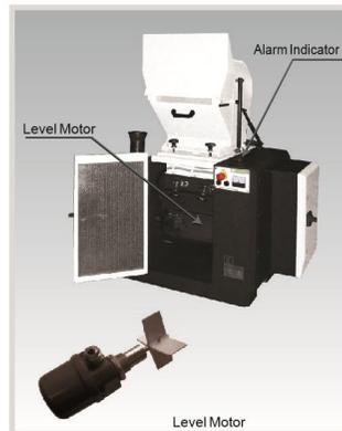
Full-receive alarm device helps to realize unmanned operation and no materials will be wasted. Whenever the regrind level reaches the motor position, the machine will be forced to stop and be cut off via its sensor, thus stop the granulator and warn the user by sounding an alarm. Add "FAD" at the end of the model code.
