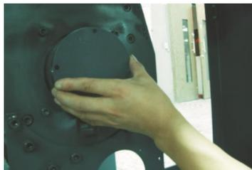
Picture 6-13: Installation of bearing cover plate
