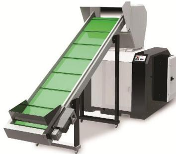
Material feeding for large granulators is quite a difficult matter. They are generally installed at a lower place or a platform must be built for material feeding. Shini particularly designed the belt conveyor to easily convey the material into the cutting chamber of SG-36 series. Add "BCF" at the end of the model code.
