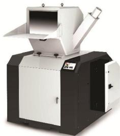
The design of feeding hopper of traditional granulators is not suitable for long pipes and section bars. We have designed material side feed pipe for convenient feeding of long materials. Add "SF" at the end of the model code.
