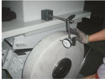
Picture 6-6: Installation of Belt Pulley and Motor 2(SG-3650)
