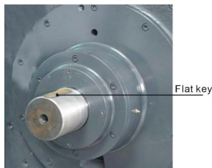
Picture 6-5: Installation of Belt Pulley and Motor 1 (SG-3650)
