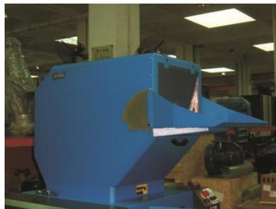
Picture 6-19: Installation of Feed Box and Feed Inletv 5
