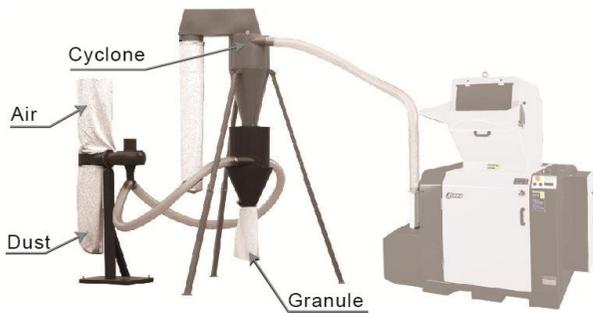
Dust Separator can separate the dust in the regrind for immediate recycle use. The dust will be kept in filter bag, thus working environment will remain clean. This device ensures full use of regrind to avoid material wasting and enhance the economy returns.
