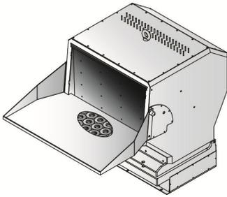
Feed hopper with magnet is used to take out metal scraps and impurities in the material. Add "FHM" at the end of the model code.
