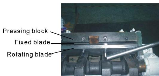
Picture 6-1: Remove The Rotating Blades
