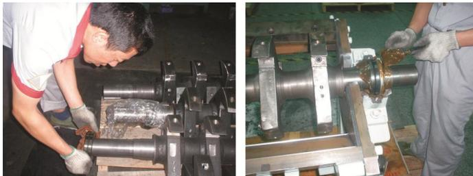
Picture 6-4: Installation of Bearing and Blade Rest
