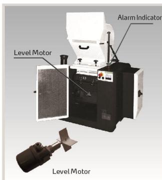
Full-receive alarm device helps to realize unmanned operation and no materials will be wasted. Whenever the regrind level reaches the motor position, the machine will be forced to stop and be cut off via its sensor, thus stop the granulator and warn the user by sounding an alarm. Add "FAD" at the end of the model code.
