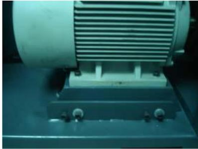
Picture 4-1: Position-adjusting Screws
