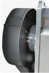
Increase inertia, thereby increasing the cutting ability. At the same time can result in a more balanced force and longer service life. Add "FW" at the end of the model code; (Option for SG-43B)
