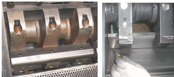
Picture 6-3: Installation of Rotating and Fixed Blade
