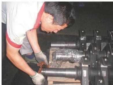
Picture 6-5: Installation of Bearing and Blade Rest
