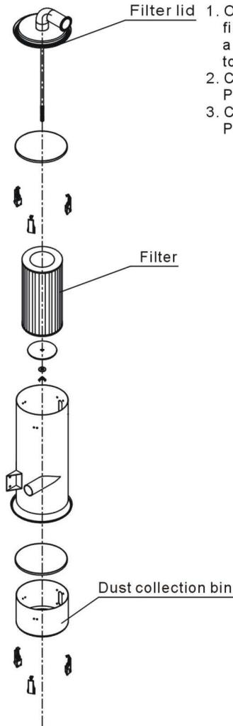
1. Open the filter lid and remove the filter, blow away the dust on it with a high pressure air gun from inside to outside.
