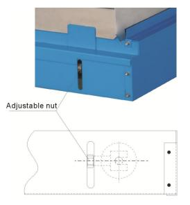
Picture 6-3: PVC Adjusting Drawing
