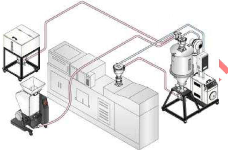
Picture 5-2: Two-stage Conveying Combination
