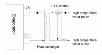
Picture 6-2: Adjusting Water Outlet Temperature by Three Way Valve
