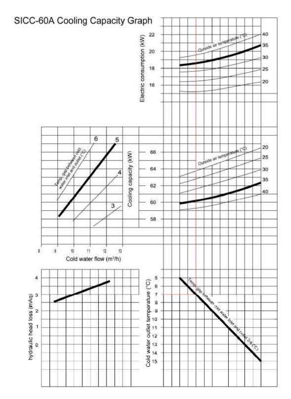
Picture 8-1: SICC-60A Cooling Capacity Graph
