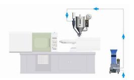
Picture 2-25: Loading With High Pressure Air
