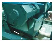
Picture 3-10: Installation of Material Storage Box 1
