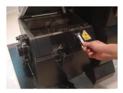
Picture 3-13: Installation of Material Storage Box 4
