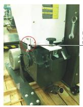
Limit block is supported on the limit sleeve
