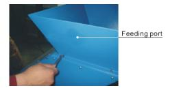
Picture 6-21: Installation of Feed Box and Feed Port 2
