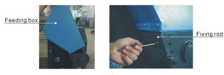
Picture 6-20: Installation of Feed Box and Feed Port 1
