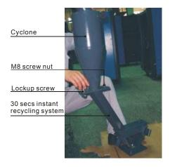
Picture 3-6: 30 Seconds Instant Recycling System 3 4) Install cloth bag at the bend place and lock it up.
