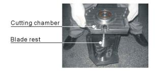
Picture 6-9: Installation of Bearing and Blade Rest 3
