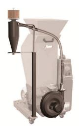
Regrind Conveying Via Blower & Cyclone (BC Type)
