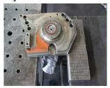
Picture 6-28: Step 1 to Take Out the Blade-rest Shaft
