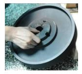
Picture 6-12: Installation of Belt and Belt Pulley 2
