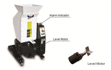
Full-receive alarm device can help to realize unmanned operation and no materials will be wasted. Whenever the regrind level reaches the motor position, the machine will be forced to stop and be cut off via it is sensor, thus stop the granulator and warn the user by sounding an alarm. Applicable to SG-16N/20N series.
