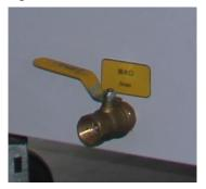
Picture 5-3: Water Drainage Port
