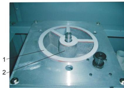
Picture 6-2: Honeycomb-rotor installation steps 1
