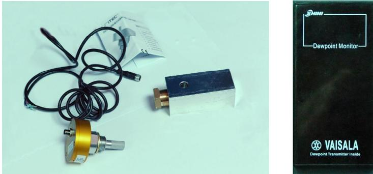
Picture 2-3: Parts of dew-point monitor
