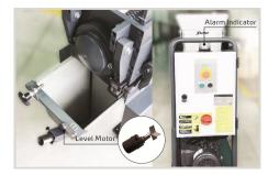
Full-receiver alarm device can help to realize unmanned operation and no materials will be wasted. Whenever the regrind level reaches the motor position, the machine will be forced to stop and be cut off via it is sensor, thus stop the granulator and warn the user by sounding an alarm.
