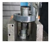
Picture 6-16: Step 1 of Bearing Dismantlement
