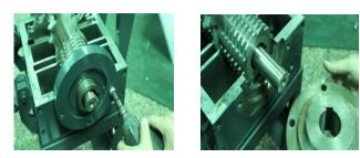
Picture 6-13: Step 1 of Left /Right Bearing Base Dismantlement
