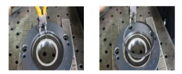
Picture 6-17: Step 2 of Bearing Dismantlement
