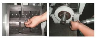
Picture 6-3: Dismantle Rotate Blades
