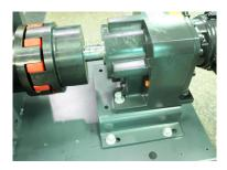
Picture 6-20: Installation of Reduction Gear 2
