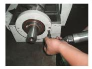
Picture 6-6: Installation of Bearing and Cutter Shaft 3
