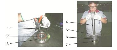
Picture 6-4: Installation of Bearing and Cutter Shaft 1
