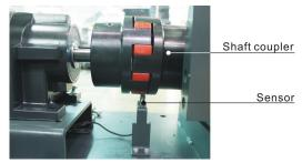
Picture 6-21: Installation of Reduction Gear 3
