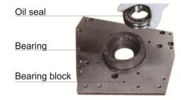
Picture 6-6: Installation of blade rest
