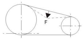
Motor of 7.5kW L=5mm F=205N For motor of 11kW L=5mm F=297N Picture 6-2: Maintenance of conveyor belt
