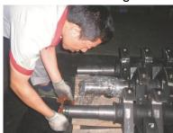
Picture 6-10: Installation of Bearing and Blade Rest
