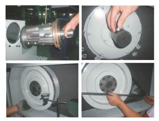
Picture 6-14: Installation of bearing, motor, belt Plley and belt
