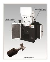
Full-receive alarm device helps to realize unmanned operation and no materials will be wasted. Whenever the regrind level reaches the motor position, the machine will be forced to stop and be cut off via it is sensor, thus stop the granulator and warn the user by sounding an alarm. Add "FAD" at the end of the model code.
