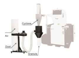
Work with cyclone dust separator to recycle the granule and separate it from dust.
