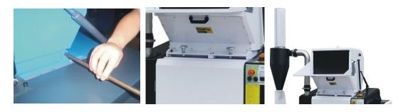
Picture 6-16: Installation of rotary blade and fixed plate (3)
