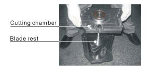
Picture 6-8: Installation of Bearing and Blade Rest 3
