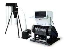
The blower stands outside the machine. Without restriction of the inner space of the machine, customer can choose different kinds of blowers.Add "SC" at the end of the model code. (Option for SG-43B)
