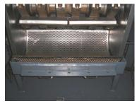
Picture 4-1: Close the Screen Bracket; the Regrind Storage Bin and the Feeding Hopper
