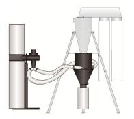
Optional dust-separating system to remove the dusts in the material.Add "DS" at the model behind.
