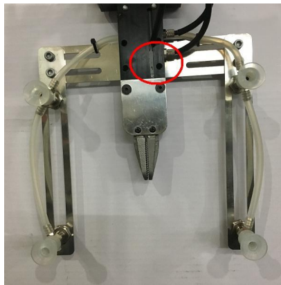
Picture 2-6: Magnetic Switch
