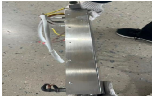
Picture 6-14: Non-contact Pipe Heater Cleaning 6
