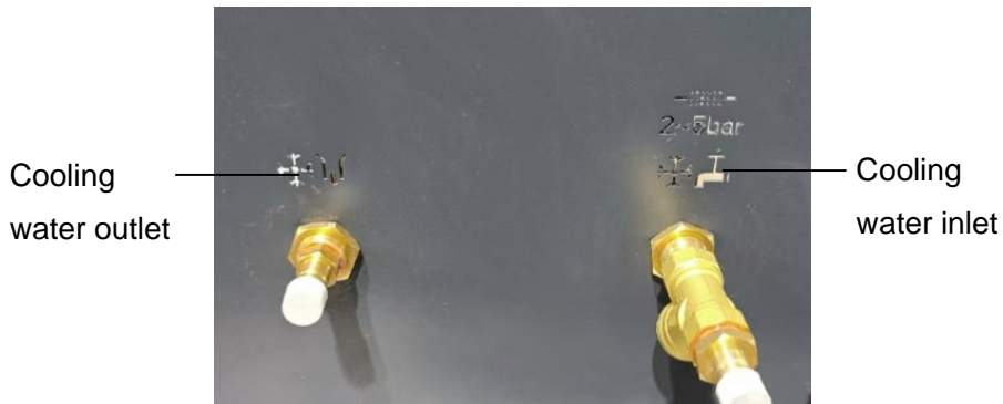
Picture 3-2: Pipe Connection
