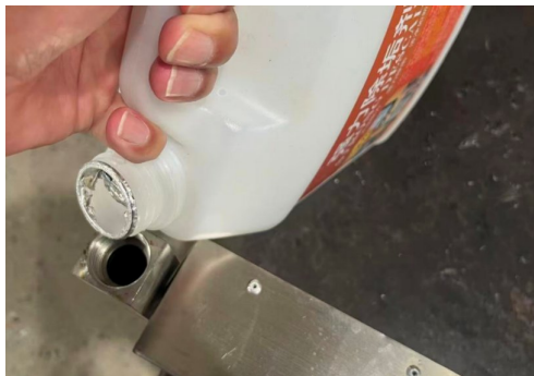
Picture 6-11: Non-contact Pipe Heater Cleaning 3
