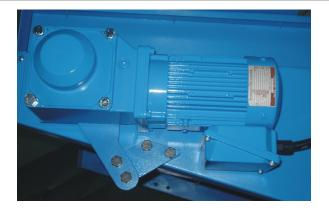
Picture 6-1: Gear Motor
