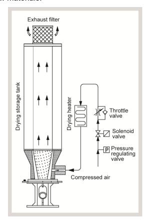
Picture 2-1: Working Principle Table (SCAD-6U and Models Below)
