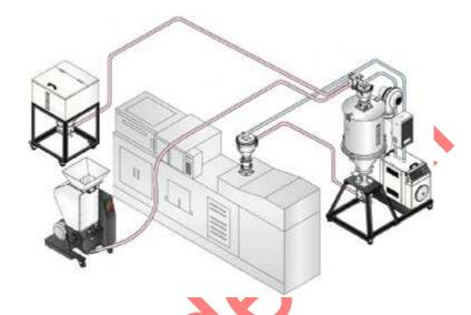
Picture 5-2: Two-stage Conveying Combination
