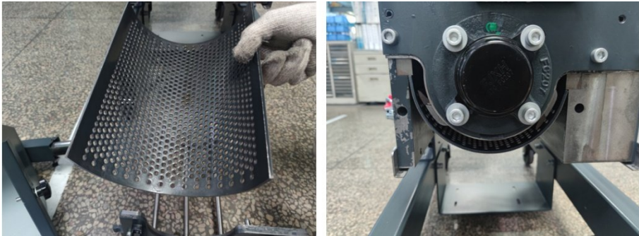
Picture 6-3: Screen and the Installation
