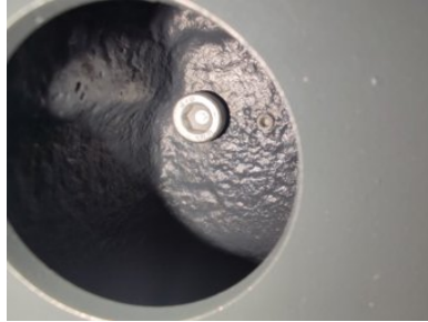
Picture 6-10: Fixed Blade Fixing Screw on the Case Block
