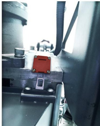
Picture 5-2: Storage Box Safety Switch Pin
