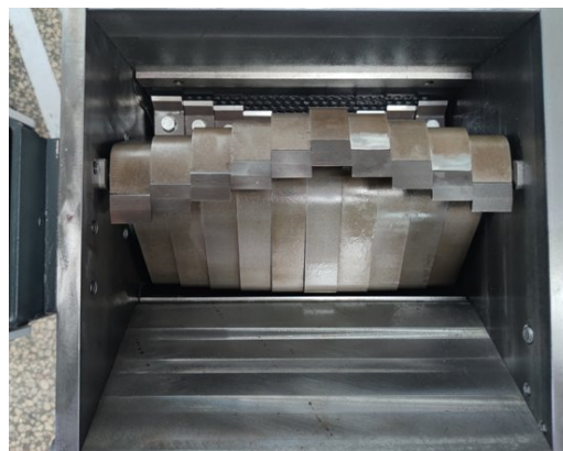
Picture 6-2: Blade Rest Installation Diagram
