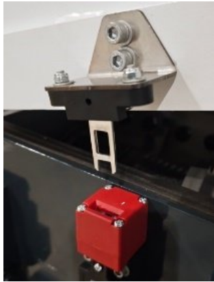
Picture 2-4: Safety Switch
