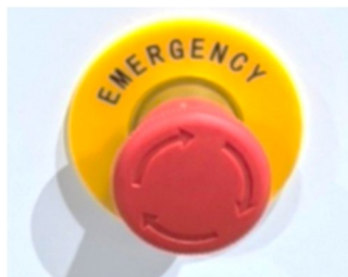
Picture 2-3: Emergency Stop Switch
