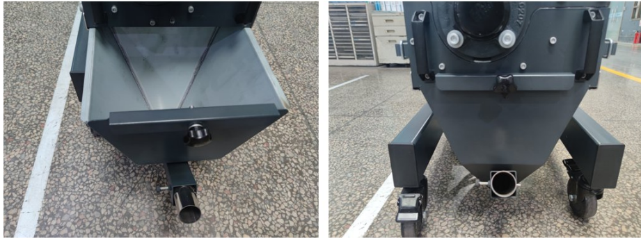
Picture 6-6: Installation of Storage Box
