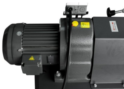
Picture 6-6: Installation of Gear Motor 3
