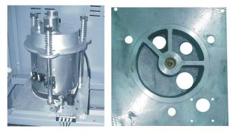
Picture 6-1: Honeycomb rotor
