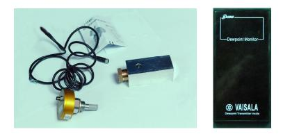
Picture 2-3: Parts of dew-point monitor
