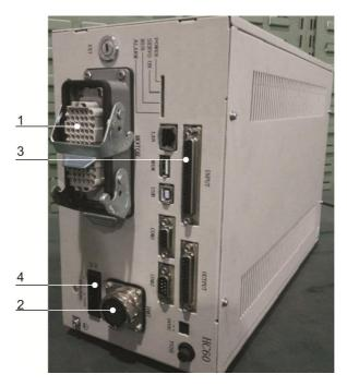
Figure 2-1: QC400 schematic side
