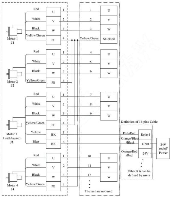
Figure 5-9: Sanyo Electric power line side wiring
