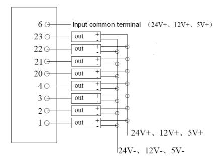
Figure 6-3: Digital input associated wiring diagram
