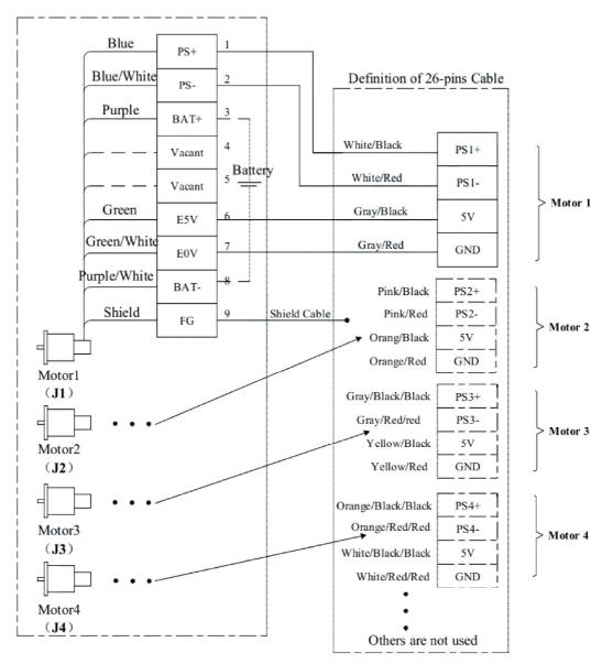
Figure 5-5: Tamagawa motor encoder line wiring
