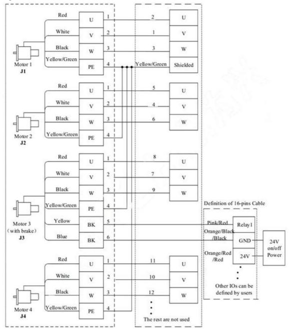
Figure 5-3: Panasonic motor power line side connection
