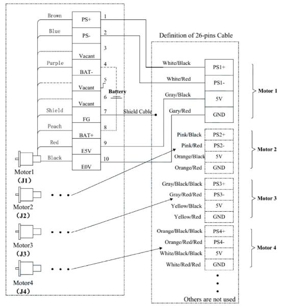
Figure 5-8: Sanyo Electric encoder wiring terminals
