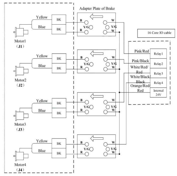
Figure 5-10: Sanyo Electric Brake side wiring
