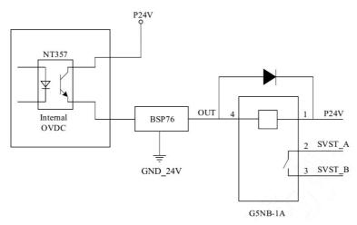
Figure 6-8: Relay Internal Connection diagram
