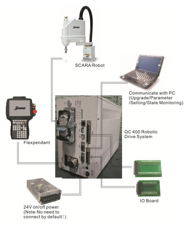
Figure 3-1: System Configuration
