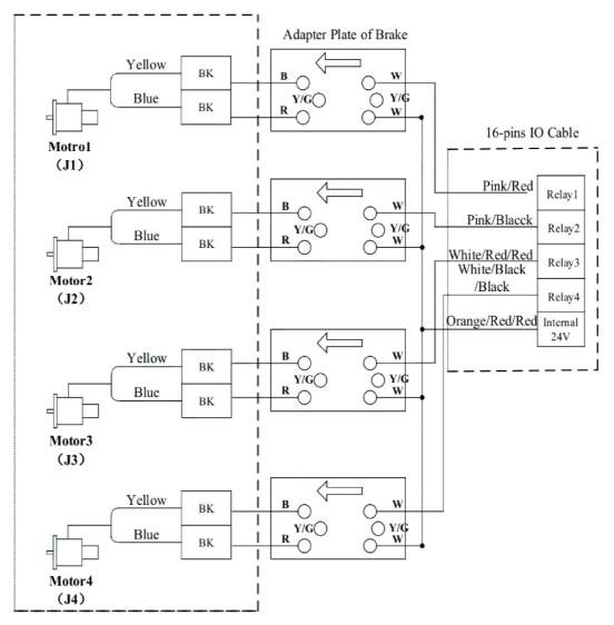
Figure 5-7: Tamagawa motor brake side wiring
