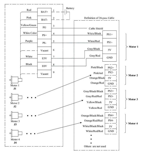
Figure 5-2: Pnasonic motor encoder terminal connection
