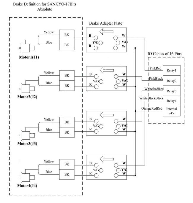
Figure 5-13: Brake Wiring of SANKYO Motor
