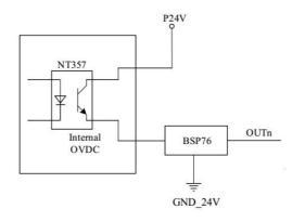
Figure 6-6: Digital output internal circuit
