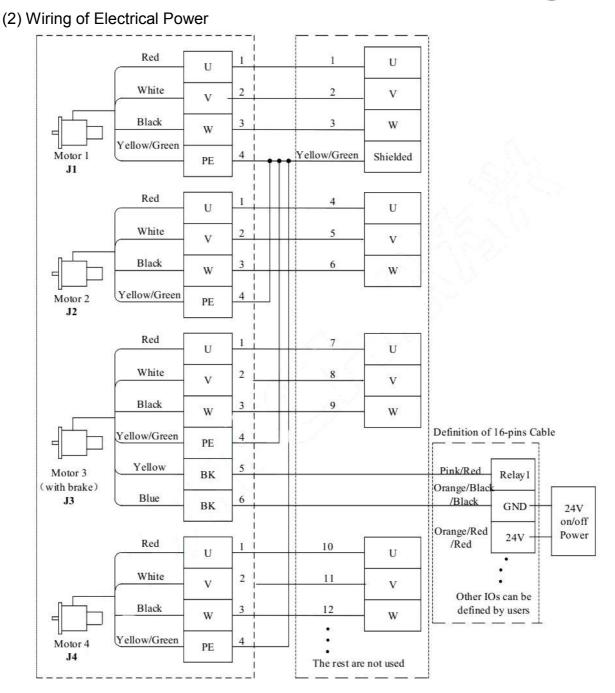
Figure 5-12: Wiring of electrical power for SANKYO
