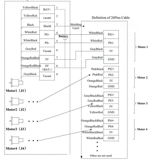
Figure 5-11: Encoder Wiring
