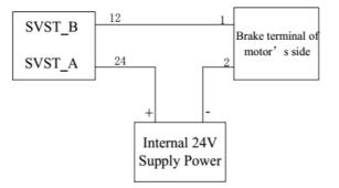
Figure 6-9: Brake-port junctions
