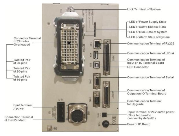
Figure 3-3: Illustrates the drive control one Terminal
