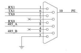
Figure 7-3: Schematic diagram of COM2
