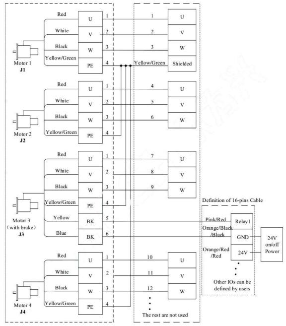
Figure 5-6: Tamagawa motor power line wiring
