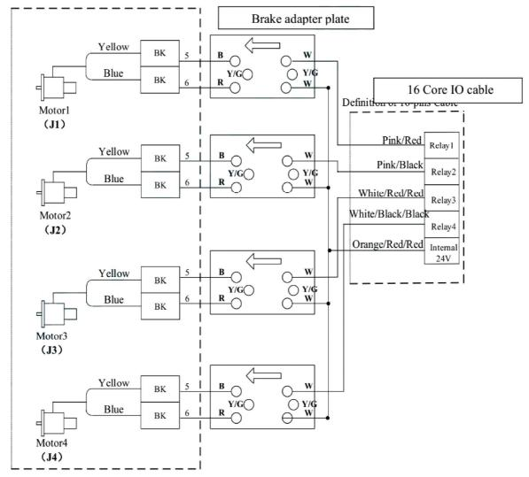
Figure 5-4: Panasonic motor brake end connection
