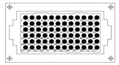
Figure 5-1: 72Pin Heavy load connector definition
