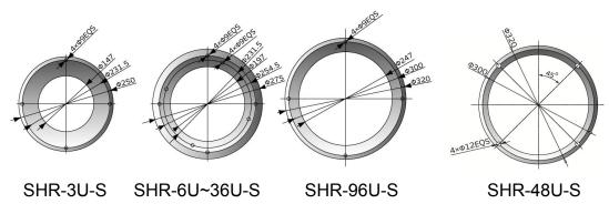
Picture 1-3: Hopper Base Installation Size
