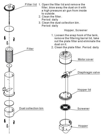
Main body, Filter Inspection and Storage Hopper Cleanup
