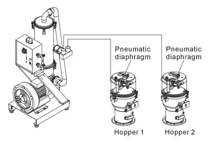
Picture 2-1: Working Principle
