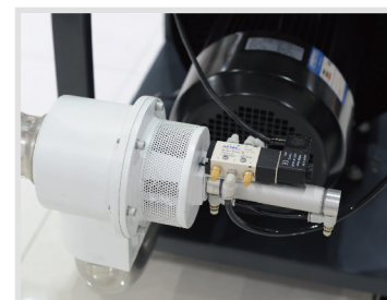
Vacuum breaking valve
